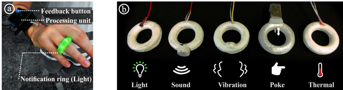
Figure 1: (a) Prototype connected to light ring; (b) Each ring supports a channel: light, sound, vibration, poke and thermal.
